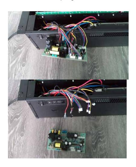
4. Plug all the wires back according to your notes or photo. Place the reattached board gently inside the unit and replace the back panel.
